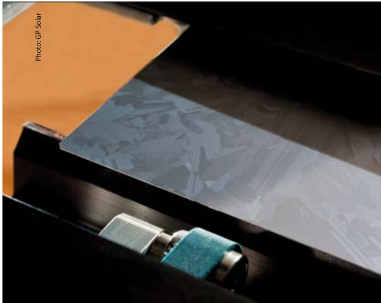
Weeding out wafers with defects is necessary to prevent unnecessary costs from incurring. Above is GP Solar's illumination concept of an in-line microcrack scanner.
