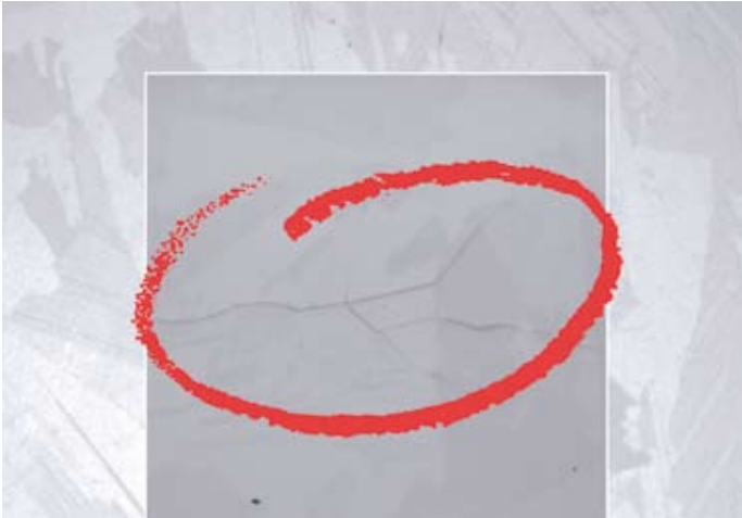
A microcrack that is detected and highlighted.
