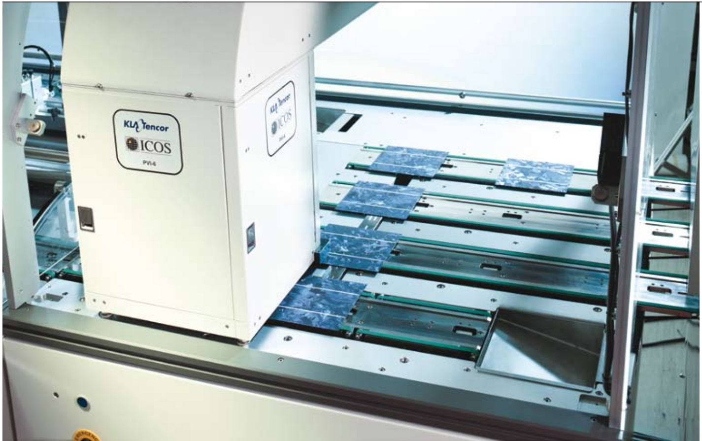
A print inspection system integrated into a screen printing machine. The system had to be designed with a 90 degree angle in order to fit into the machine's housing.
