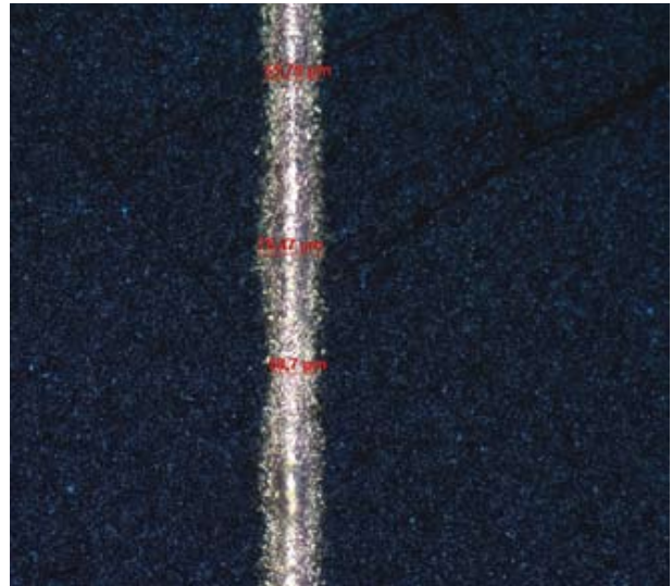
Details of a grid finger as seen by an optical inspection system. Writing software algorithms for producing a sensible reading for the finger width requires a good understanding of the printing process.
